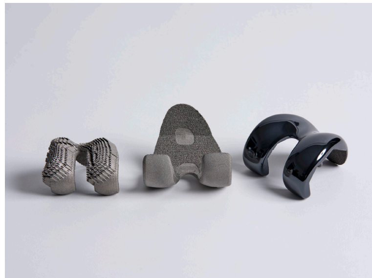
Femoral components in multiple stages after 3D printing: with print supports, without print supports and fully finished with an anti-wear ceramic bearing surface.
