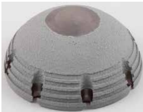
Figure 3: HA coating applied to acetabular cups.
