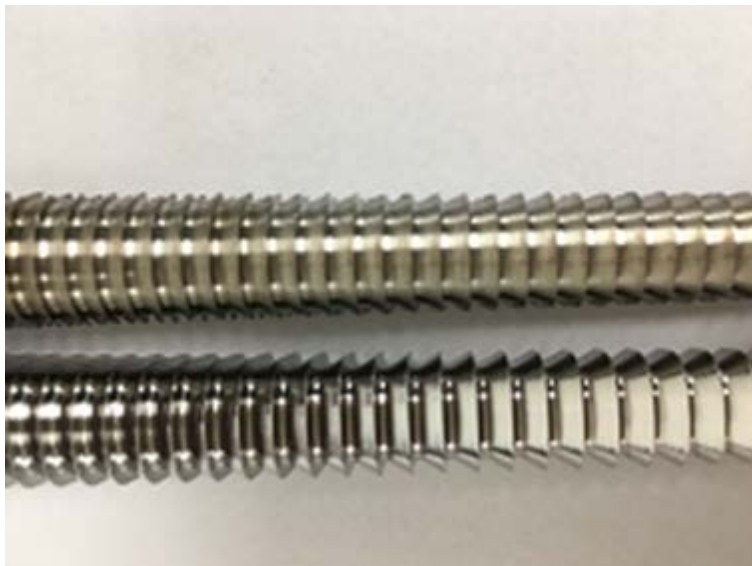
Figure 10 – Photograph showing discolouration of wrought product at 11 autoclave cycles and Orchid product maintained polished surface after 40 autoclave cycles
