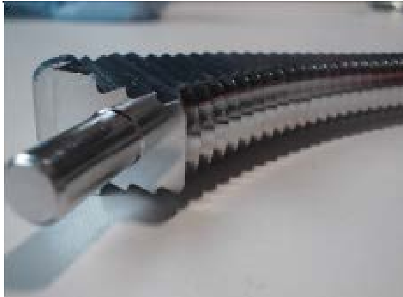
Figure 9 – Orchid Broach product after Salt Test
