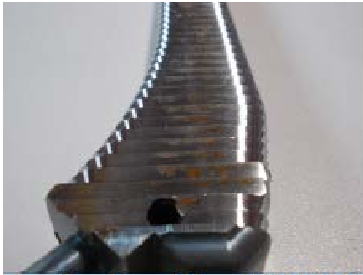
Figure 8- Standard wrought broach showing evidence of Pitting corrosion
